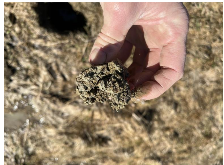
Photo 4. A representative soil sample, showing prominent redoximorphic features, from the mowed portion of Wetland A
